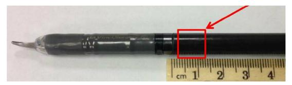
According to the notice: "These micro-cracks may <u>not</u> be visible to the [surgeon]." And according to the notice, the issue is significant because: "This may create a pathway for electrosurgical energy to leak to tissue during use and potentially cause thermal injury."
